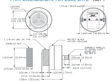
NOTE A: TERMINALS -0.32 BRASS TIN PLATED, TAPPED FOR #6-32 SCREW, TWD #6-32 NICKEL PLATED BRASS SCREWS INCLUBED, WILL ACCEPT 1/4" QUICK CONNECT.
